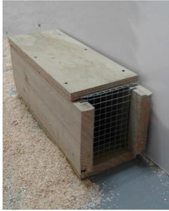
**Figure 5. The Predator Free NZ wooden trap tunnel used for tests 5 and 6. A 50 × 50 mm entrance hole was cut in the mesh at the far end of the tunnel (not visible) and the mesh at the closed end of the tunnel was removable to allow access to the trap. The T-Rex trap was set 2 cm into the tunnel from the closed end. Two tacks were nailed into the trap tunnel floor in front of the trap to prevent it being pulled forward, or pushed too close to the entrance hole in the front mesh.**
