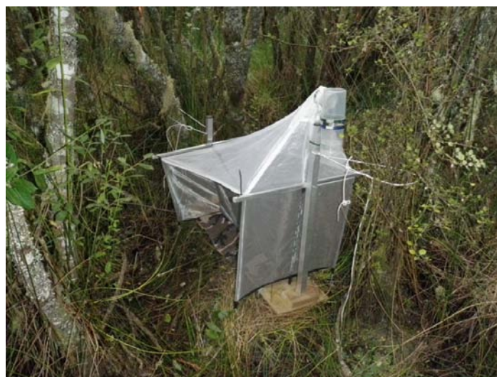
One of Corinne's malaise traps set up at Whangamarino for sampling invertebrates
