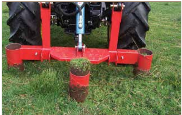
Planting can be dramatically sped up with this novel hydraulic hole-puncher which pulls PB3-sized plugs out of the ground. Photo: Alec Bennett, Lake Cameron Care Group
