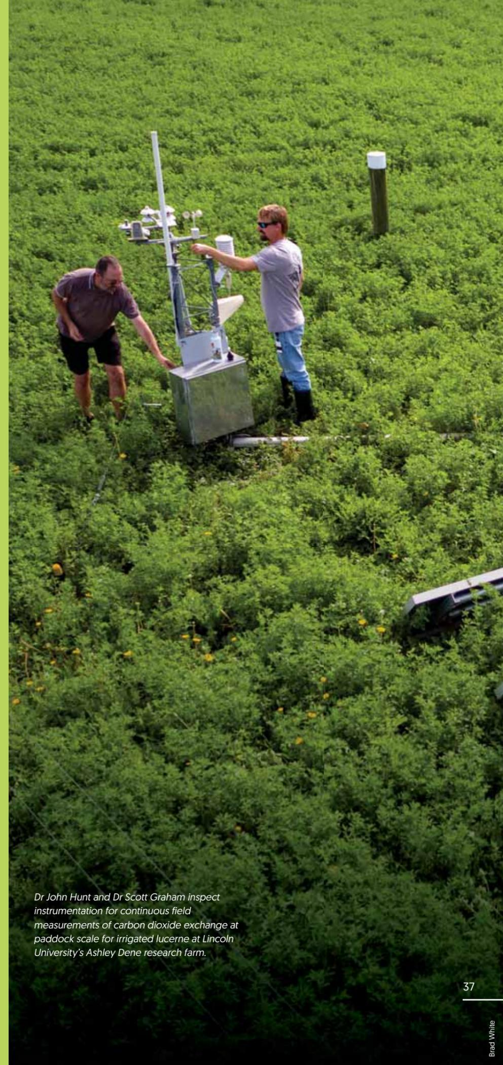
Dr John Hunt and Dr Scott Graham inspect instrumentation for continuous field measurements of carbon dioxide exchange at paddock scale for irrigated lucerne at Lincoln University's Ashley Dene research farm.
