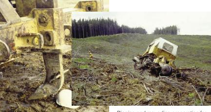
Ripping and mounding preparation for planting at Riverhead Forest, Auckland (15%) with mounding and ripping of the Densipan Ultic Soil.
