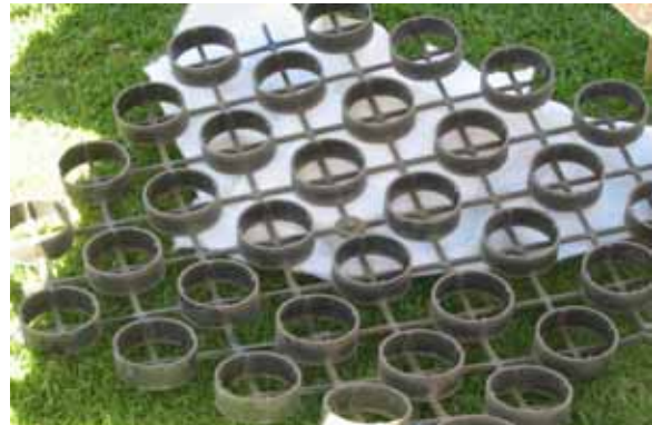
Figure 30 (a) and (b): Strong plastic grids increase bearing strength, reduce compaction of substrate, and allow plants to grow. Melbourne, Australia. Photos: Marjorie van Roon
