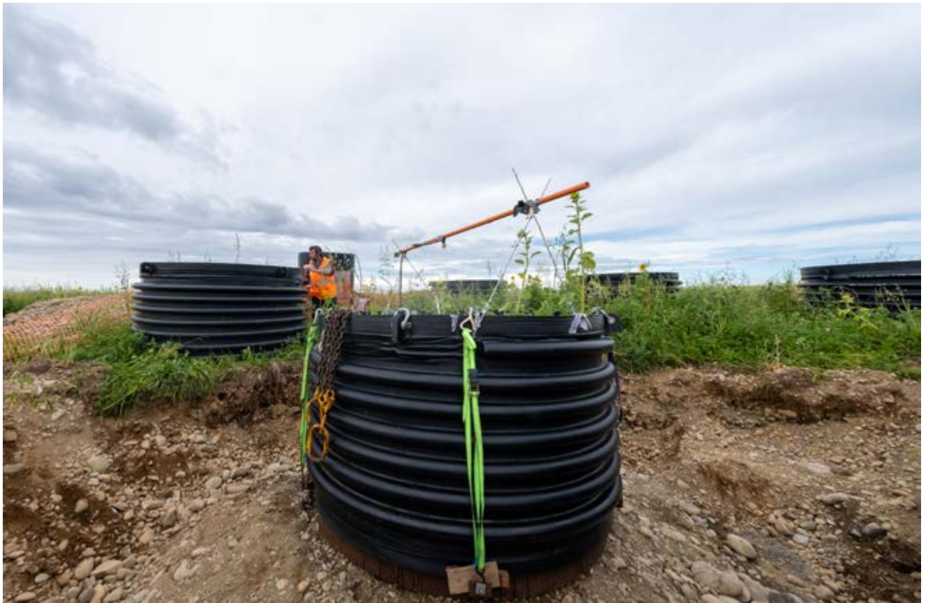
The installation of the lysimeters deep into the fields on the Canterbury plains.
