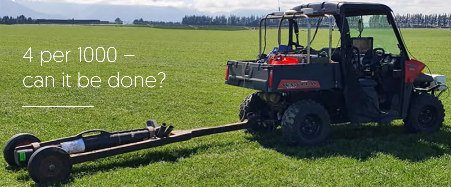
Non-invasive proximal soil sensing digital data acquisition instruments in action on the Lincoln University dairy farm.
