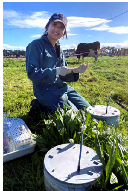
Chi Vi collecting gas samples to measure nitrous oxide emission from plantain treatment plots.
