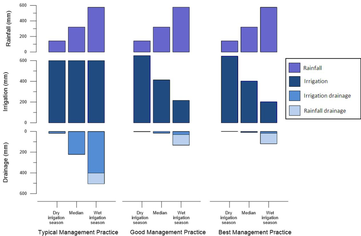
Figure 4. Total rainfall (mm), total irrigation (mm), and total drainage (mm) under TMP, GMP and BMP. Dry, wet and median seasons are based on the amount of rainfall received during the irrigation season. See Box 2 for modelling details.
