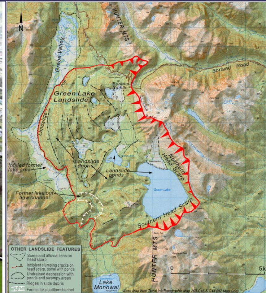
Left, the Taihape landslide (Massey, 2010). Right, topographic map of the Green Lake Landslide (Hancox & Perrin, 2009)
