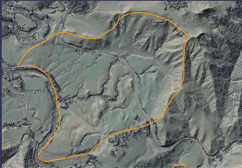
Example of an “Old” Landslide
