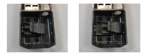
Figure 4. Unset T-Rex rat trap in an open Sidekick bait station. *Left:* Trap placed fully back in the trap recess so that rats had access to the front edge of the trap, as used for test 3. *Right:* Trap placed forward in the trap recess so that the leading edge of the trap was flush with the wall of the bait station. This set was used for test 4.
