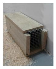
Figure 5. The Predator Free NZ wooden trap tunnel used for tests 5 and 6. A 50  $\times$  50 mm entrance hole was cut in the mesh at the far end of the tunnel (not visible) and the mesh at the closed end of the tunnel was removable to allow access to the trap. The T-Rex trap was set 2 cm into the tunnel from the closed end. Two tacks were nailed into the trap tunnel floor in front of the trap to prevent it being pulled forward, or pushed too close to the entrance hole in the front mesh.
