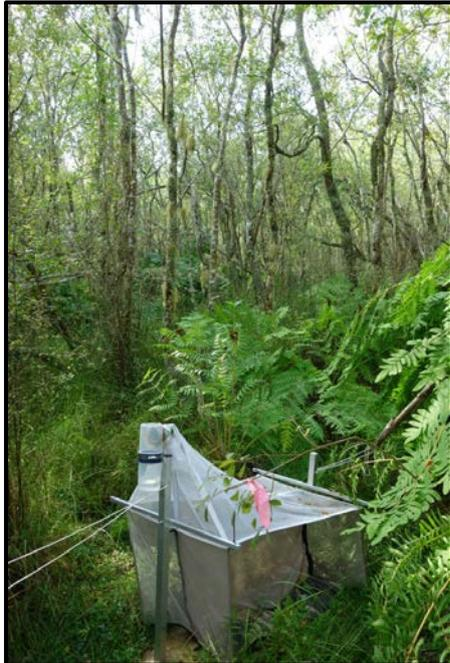
A malaise trap for sampling invertebrates, in an unsprayed plot in Whangamarino wetland. Photo: C Watts.
