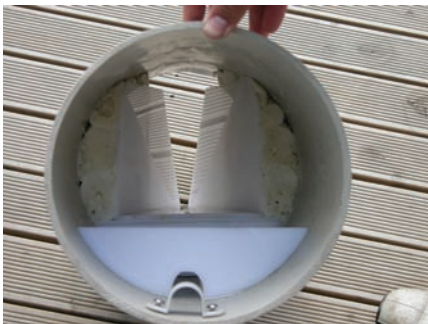
The flume that measures flow from the base of the raingarden. Topsoil spread.
