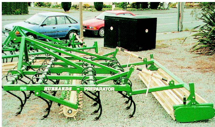
The preparator 1 – a one-pass cultivator with two sets of double-row Danish mixing tines, a front roller and a bar crumbler at the rear
