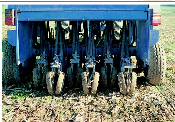
Modern coulters designs have eliminated many of the problems associated with early no-till drills
