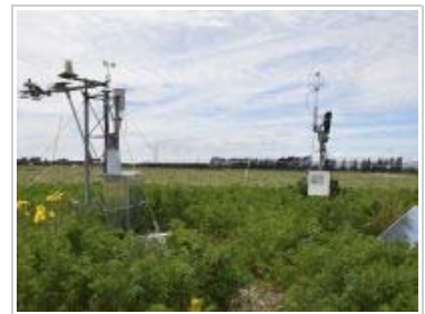
Figure 1. Measurement site in irrigated lucerne field, with weather station on left and CO 2 -exchange instrumentation on the right. The lucerne around the site has just been harvested, and the vegetation left standing is about to be cut by our team to determine the biomass-carbon accumulated since the previous harvest. (Photo: John Hunt)
