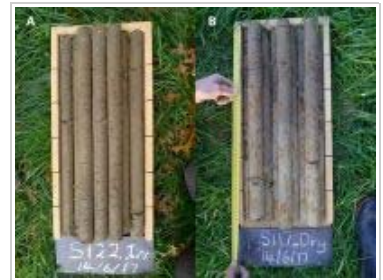
Figure 1. Soil cores from a Recent (A) and Pallic (B) Soil in the Wairarapa.
