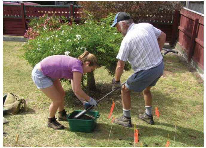
FIGURE 1 Sampling soils under a greywater application site onto a household lawn.
