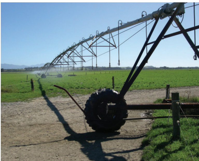
Figure 1: A variable rate irrigation system can shut off water as it passes over a farm track.
