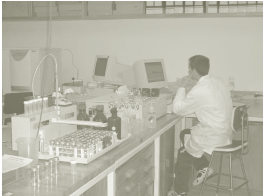
The Lachat FIA analysing leachate samples
