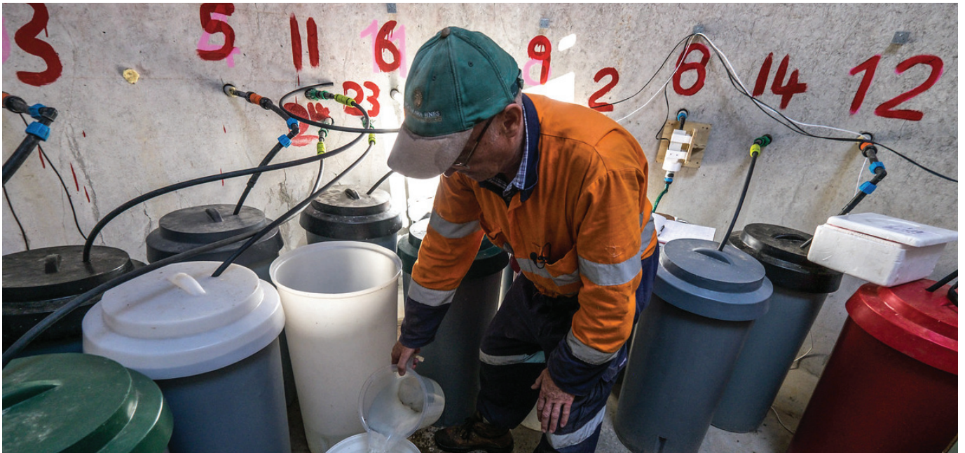
Malcolm McLeod measuring the waste collected from the large lysimeter on the farm in Tihoi.
