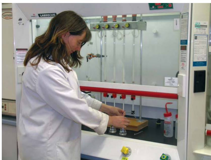
The gel permeation chromatography system used to 'clean' samples.
