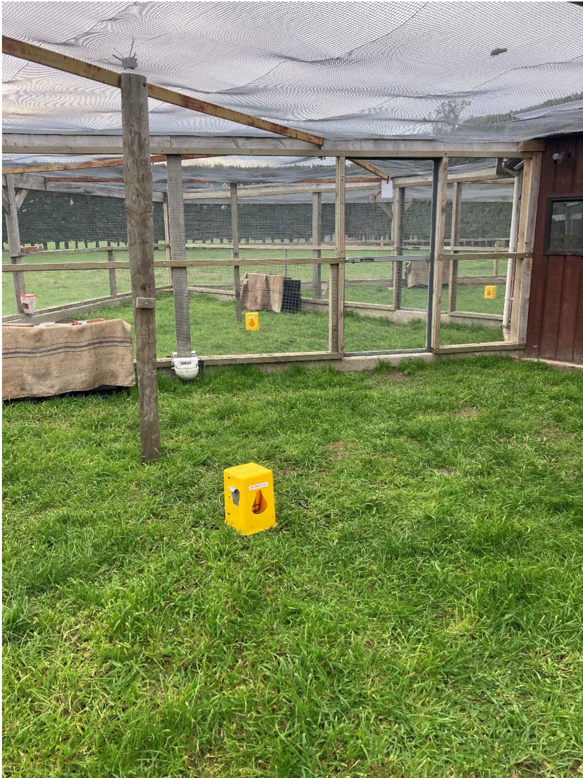
Figure 7. Timms traps deployed in observation pens. The traps were firmly secured to the ground using the pins provided with the trap. A circular 55 mm hole, duct-taped back in place, was cut in the side of the trap so that time to loss of palpebral (blinking) reflex) by captured possums could be assessed.
