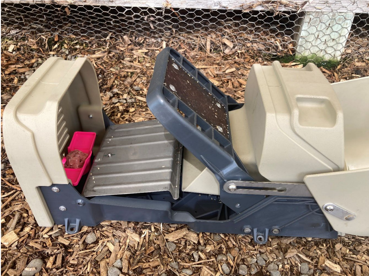
Figure 2. Open Rewild kill trap. The trap was baited with chicken mince placed in the bait well of the trap. The top cover is attached to the kill bars, so opening the cover raises the kill bars and disengages the treadle, putting the trap into safe mode for baiting. (See https://rewild.nz/wp-content/uploads/2022/12/Quick-Start-guide.pdf , accessed 7 March 2023).
