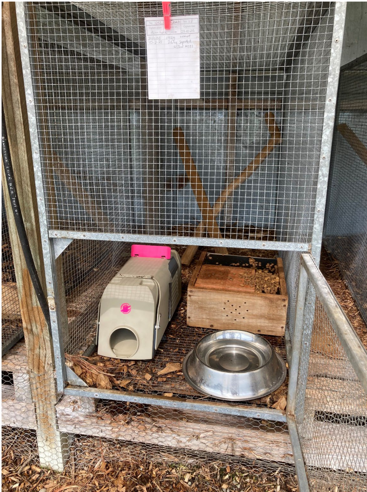
Figure 1. Unset Rewild kill trap in a stoat cage next to a stoat nest box. The raised pink flag on top of the trap indicates that the trap is unset or has fired. The trap was baited with chicken mince placed in the bait well of the trap, located behind the trap treadle at the rear of the trap (not visible).
