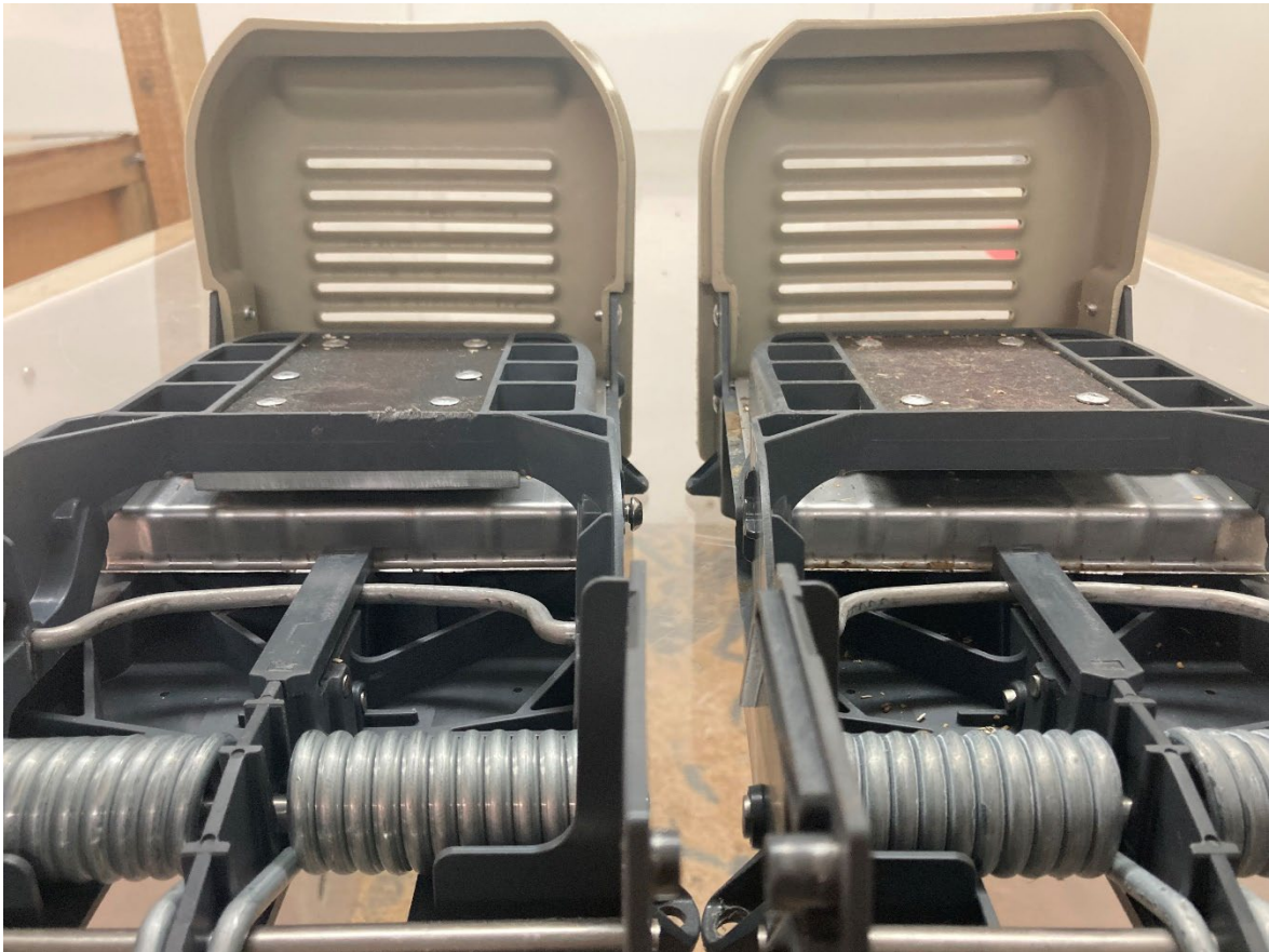
Figure 4. Extension to kill bar (L) compared to original Rewild trap (R). This reduced the gap between the treadle and kill bars when the trap fired, and this configuration was used for the third trial of Test 3. The top cover and entrance chamber have been removed to provide a view of the difference. Trap kill bars are shown in fired position.
