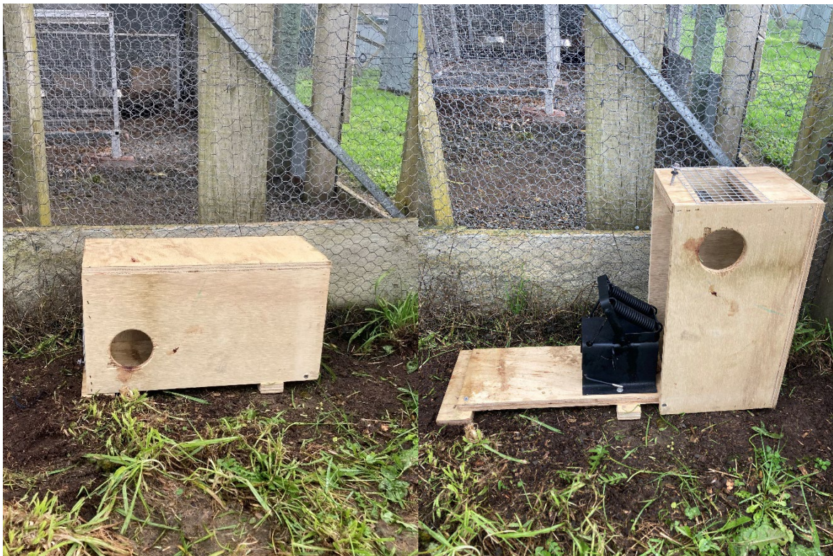
Figure 8. SA4 trap deployed in an observation pen. The trap tunnel has mesh front and rear and 70 mm diameter entrances on each side (L). The tunnel cover was secured with a hex head screw to the base. The screw was loosened to pivot open the tunnel cover (R) to access the trap and assess captured ferrets. The trap was baited with a cube of rabbit meat secured on a bait spike at the rear of the trap (not visible).
