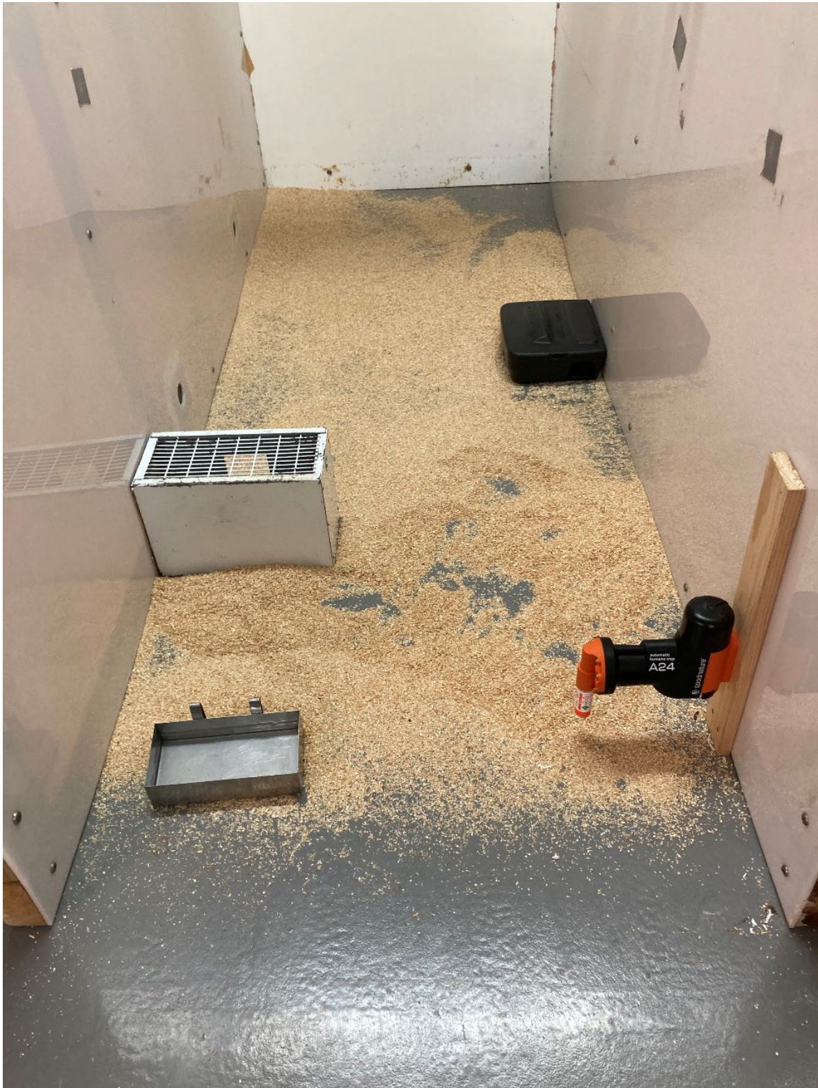
Figure 6. A set Goodnature® A24 trap deployed in a test arena. The trap is screwed to a vertical board, with the base of the trap 12 cm above the ground and baited with the chocolate-based rodent paste deployed in an automatic lure pump as per the manufacturer's instructions. A Protecta EVO Ambush bait station (in background) was provided as a secondary nest box.
