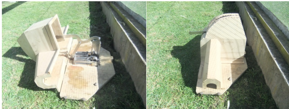
Figure 1 pT1000 kill trap in double-ended tunnel. L: Tunnel opened to show trap. R: Tunnel closed. Six rebar rods were used to pin down the trap tunnel base. Trap and tunnel shown is the final configuration, which is unset in both photos. The trap was firmly bolted to the tunnel base.
