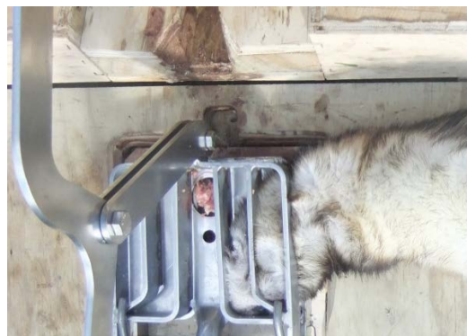
Figure 4 The position of bait used with the podiTRAP™ during test 6 for capturing ferrets. Bait was placed in a trough in the centre front of the trap. The tunnel is shown hinged open.
