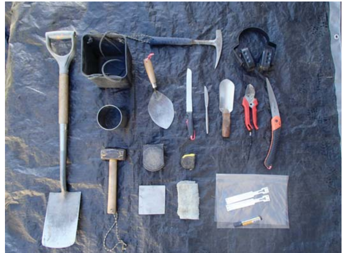
FIGURE 2 Equipment required to deal with the various issues encountered when collecting soil bulk density soil samples in plantation forests
