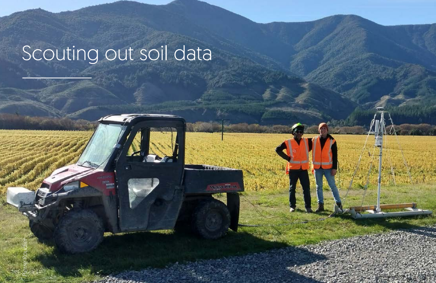
Marlborough District Council environmental science technician Zeke Hoskins (right) and Manaaki Whenua – Landcare Research technician Kishor Kumar (left) standing next to the mobile soil-sensing platform.
