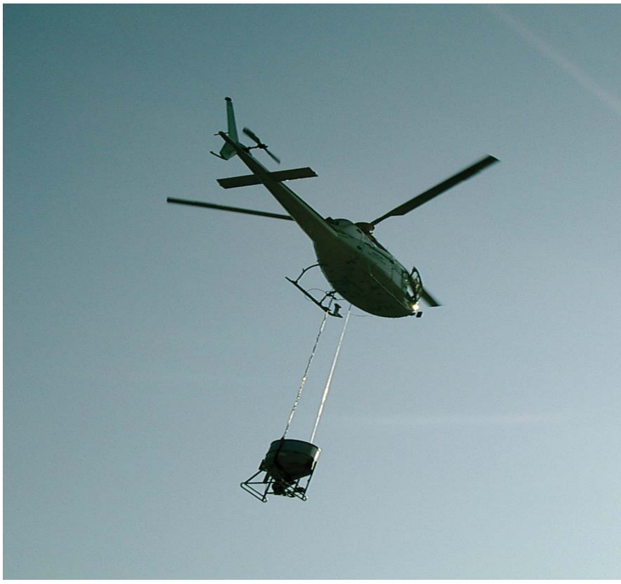
The modified sowing bucket in use at Molesworth.
