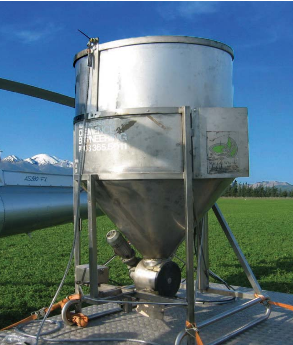
The SowLow bucket modified with a gated paddle wheel mechanism for aerial delivery of bait in clusters as used in the Landsborough and Molesworth trials.
