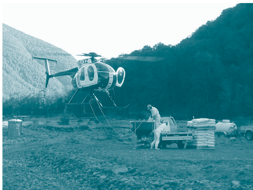
Filling a sowing bucket with 1080-loaded cereal bait prior to aerial delivery.
