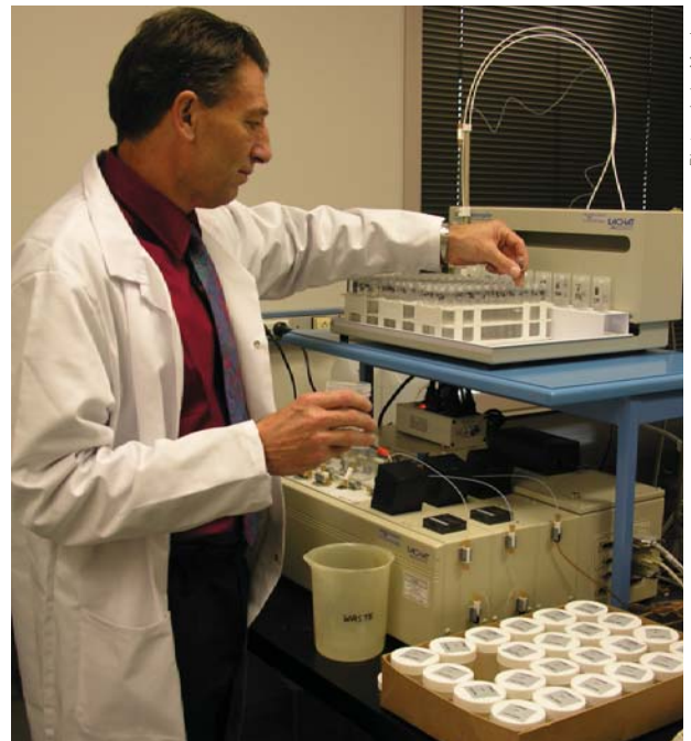
FIGURE 2 Measuring nitrogen and phosphorus in river water samples from the NRWQN on the Flow Injection Analyser (FIA) in NIWA Hamilton's water quality laboratory.
