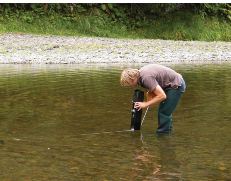
FIGURE 1 Measuring visual water clarity at a river site in the NRWQN. The technician is using an underwater periscope (black item in his left hand) fitted with a 45 degree mirror to view horizontally under the water surface. Visual clarity is the distance (measured by tape measure) at which the visual target (black disc on the left of the image) disappears. The black disc is fixed to a steel pole driven into the river gravel.
