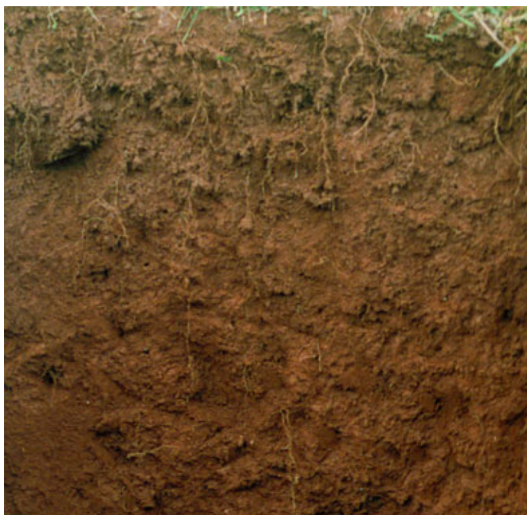
Figure 12. Soil with good porosity because of weak strength and good aggregation. There is wide distribution of soil pores sizes, from large pores between fine aggregates (peds) that enable drainage of water and entry of air to roots, and fine pores within aggregates that provide good water storage.
