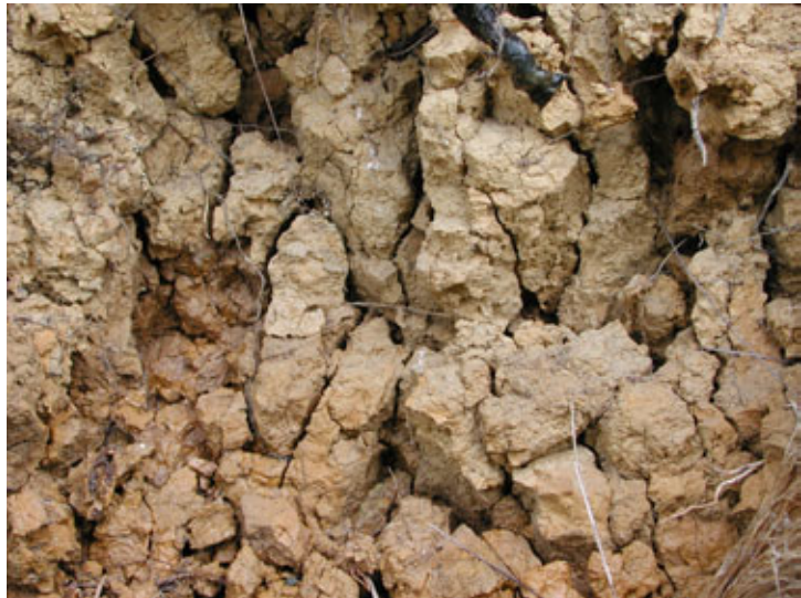
Figure 13. Strongly developed soil structure in the subsoil of a clayey ancient soil (Ultic Soil) in Northland. The structure comprises blocky aggregates (peds) with large open pores spaces between them. The roots indicate scale.
