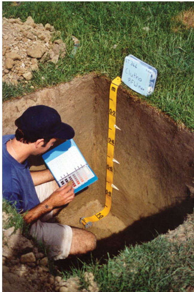
Figure 1. The ultimate soil pit dug deep and wide to provide an excellent view of soil layers. The soil scientist is measuring soil colour using a soil colour chart.
