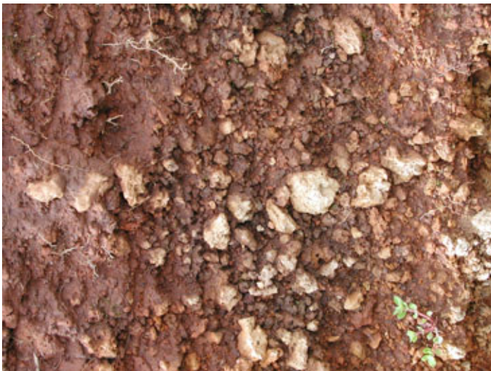
Figures 11. Stones in the form of scoria in a soil formed from weathered basalt at Mt Wellington, Auckland. The scoria dilutes the volume of soil available for storage of water and for roots to extract nutrients. In a wet climate however, water storage is not as critical as in a dry climate. The material between the stones is loose and water is able to drain, and roots penetrate easily through it.
