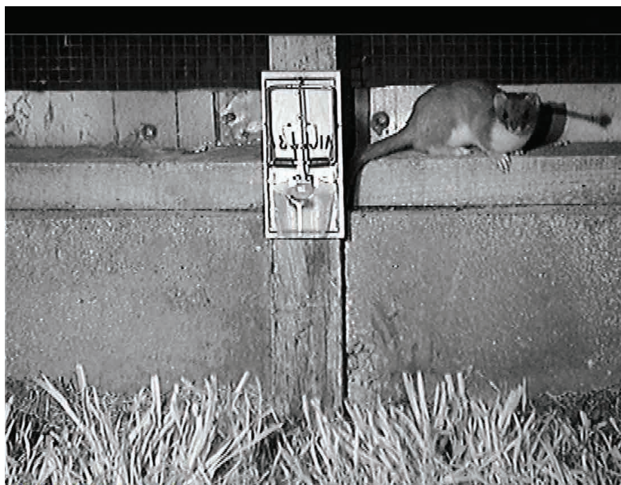
Testing modified Victor Easy Set rat trap on stoats.
