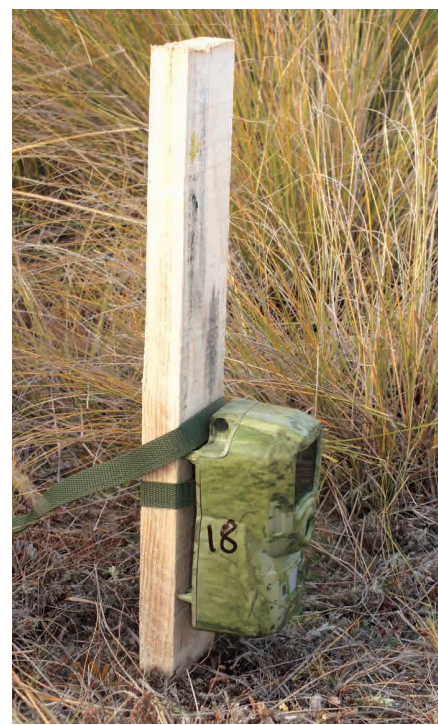
Camera-trap set up to monitor predators.
