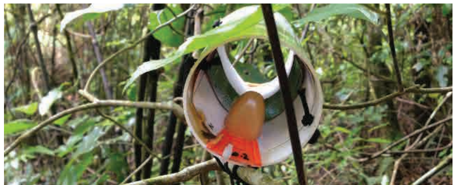
Researchers developed this chew tag and tracking device that can be pulled up into the canopy to study mouse climbing.
