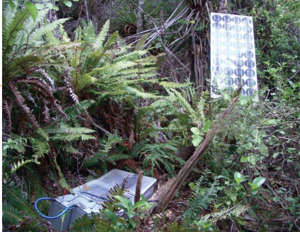
The scanner and data logger in a waterproof box and linked to a solar panel for continuous operation.
