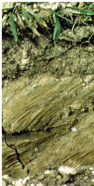
FIGURE 3 Anthropic Soils profile formed on a sports field where soil material has been transported on the site and compacted by heavy machinery.
